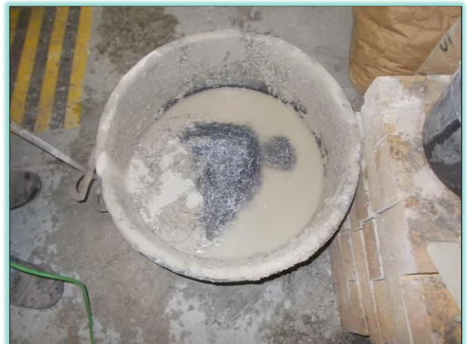
Fireproof castable reinforced with stainless steel fibers (heat resistant)
